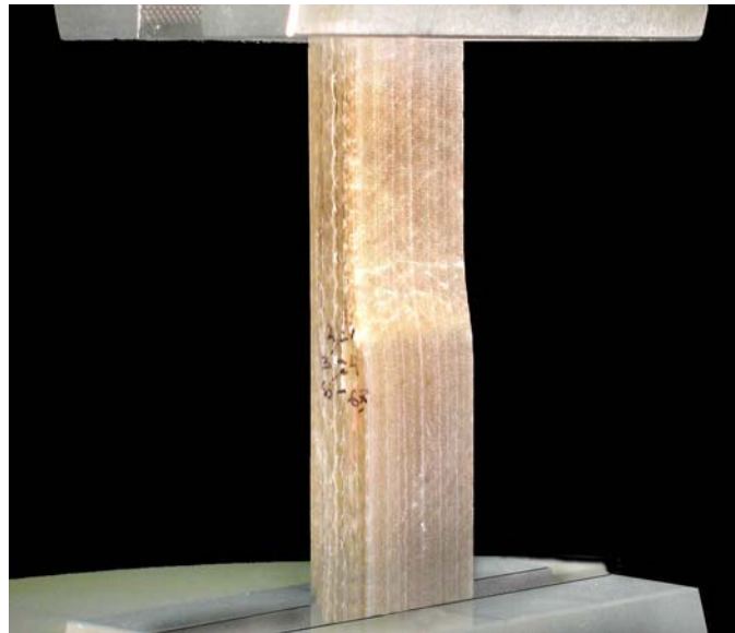
Figure 23. MSU complex coupon with fatigue damage at ply drops, VE-2 resin.
