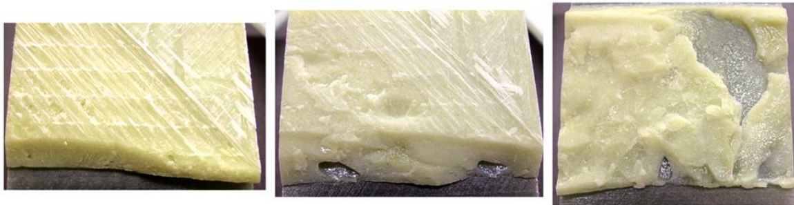
Figure 117. Fracture surfaces of Geometry A specimens, Point A, Figure 29 is at the bottom of the adhesive in each case, with crack propagation toward the top. Left, stronger than average specimen, no major flaws; center, weaker specimen, two large pores along edge of adhesive; right, weakest specimen, poorly cured adhesive (cohesive mode over entire surface).
