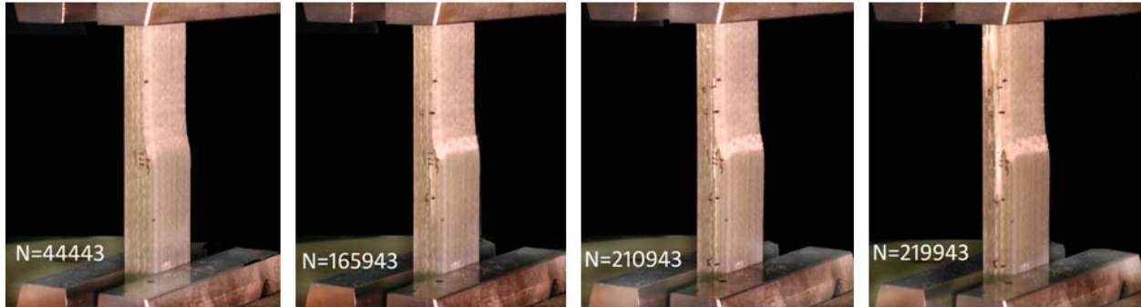
Figure 84. Images of damage in complex coupon with VE-1 resin, two ply drops, maximum load 44.5 kN, R = 0.1 , at four cycle levels, N = 44443, 165943, 210943, 219943 .
