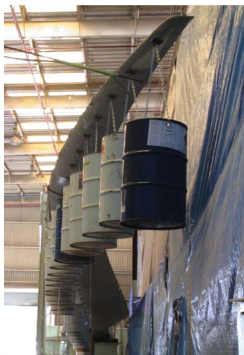
Figure 2.11 Barrel testing the prototype blade to verify twist under load.
