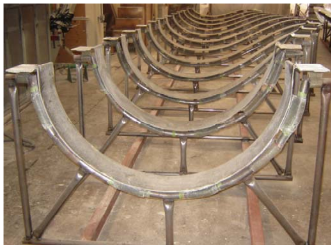
Figure 2.8 Assembly fixture for holding the blade shells during final bonding.
