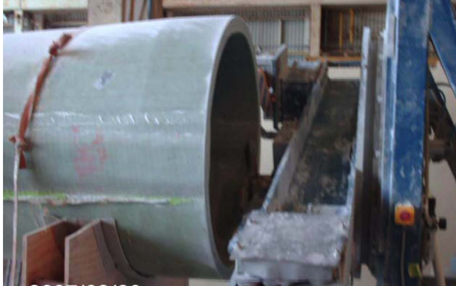
Figure 4.13 Photograph of the blade root drilling for T-bolt fasteners.
