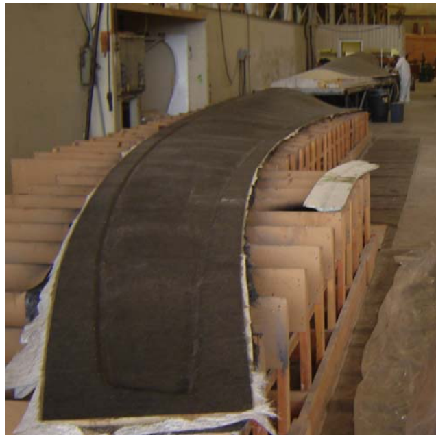
Figure 2.6 Laminating over the finished pattern for the STAR blade.
