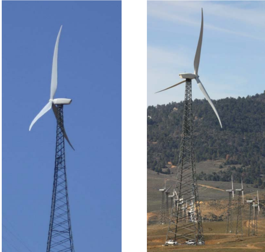
Figure 2.12 STAR prototype blades on the Zond 750 test turbine in Tehachapi in April 2008.
