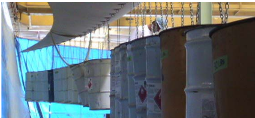
Figure 2.10 Barrel testing the prototype blade to verify twist under load.
