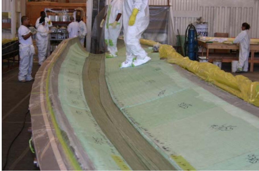
Figure 2.9 Fabrication of the STAR 54 field test blades in South Dakota.
