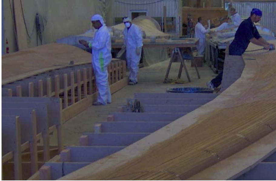
Figure 2.5 Workers smoothing the STAR blade pattern.
