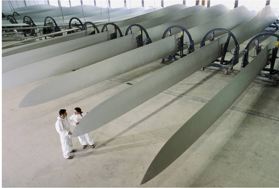
Figure 4.14 Large wind blades in the finishing hall (LM Glasfiber photograph).
