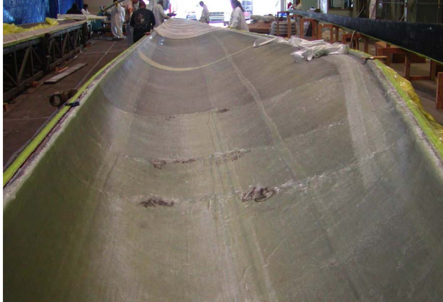
Figure 4.7 Photograph showing outer skin laminations in the blade mold.
