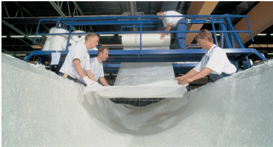
Figure 4.10 Placement of dry fabric in the blade shell mold (LM Glasfiber photograph).
