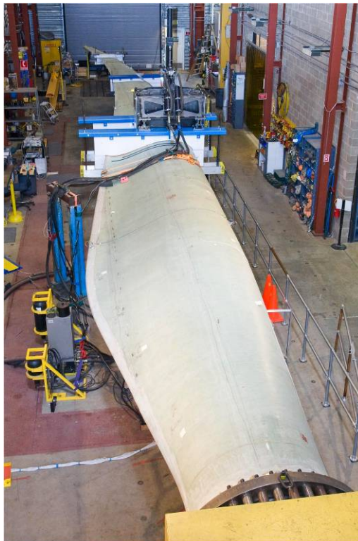
Figure 6.18 STAR prototype blade in NREL test stand with loading saddles.
