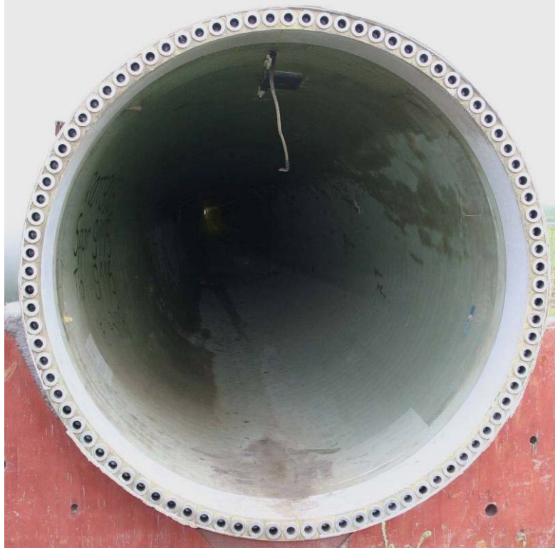
Figure 3.2 Root view of spar-shell blade with bonded threaded inserts.
