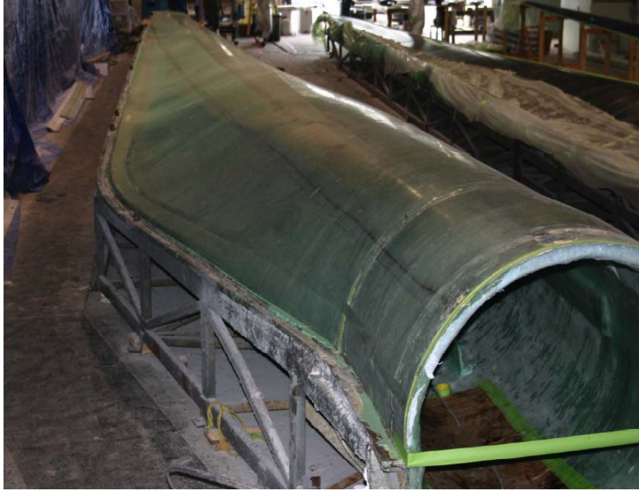
Figure 4.12 Photograph of a cured blade during the demolding process.
