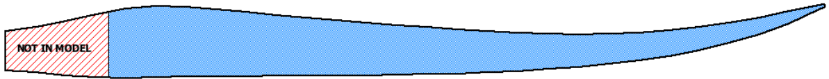
Figure 5.33 Illustration of the root region not included in the finite element model.
