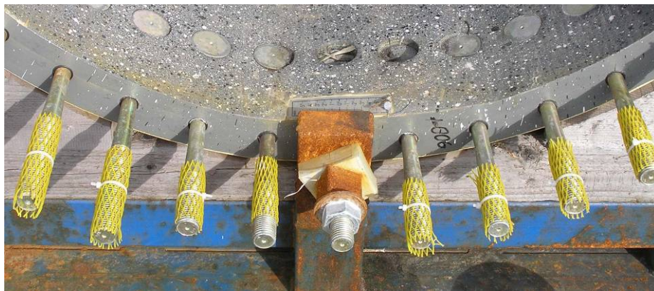
Figure 3.11 EuroS EU-51 blades with T-bolt type root attachment.
