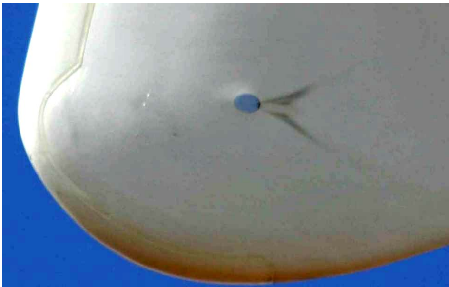
Figure 3.12 Blade receptor after a lightning strike showing burn marks, but no damage.
