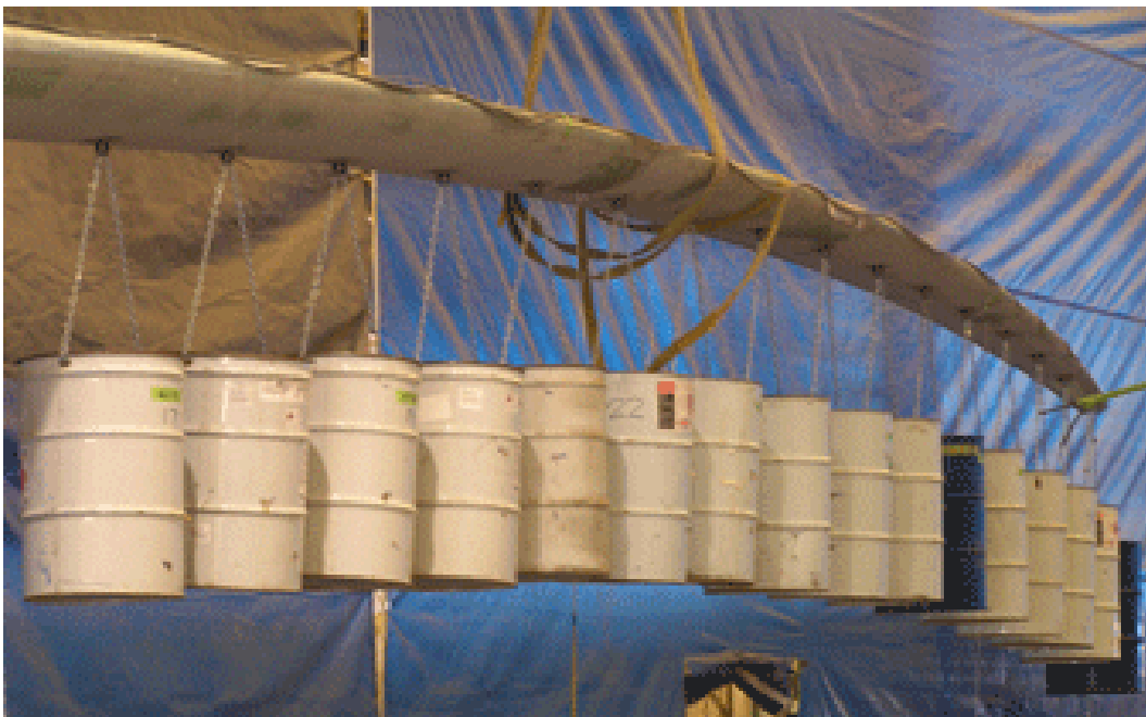
Figure 6.12 Blade loaded with water barrels.
