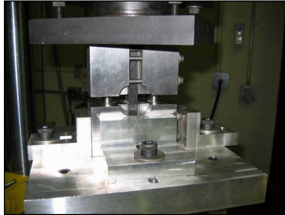
Figure 5-14. D6641 (CLC) Thick-Coupon Test Fixture
