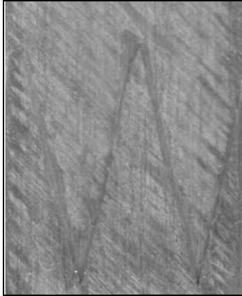
Figure 5-21. Face View of Prepreg Pinked Ply Termination
