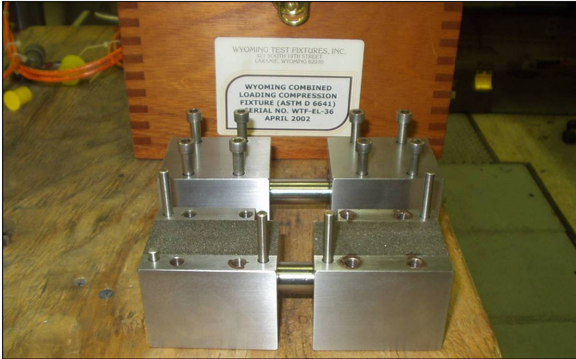
ASTM D6641 Test Fixture at WSU
