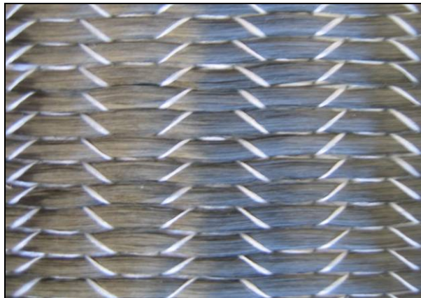
Figure 4-1. Stitched Fabric with Manufacturing-Induced Waviness
