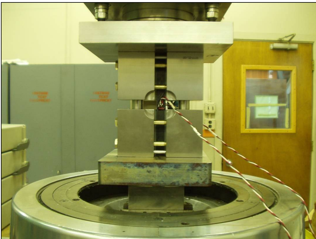
ASTM D6641 Test Setup at WSU
