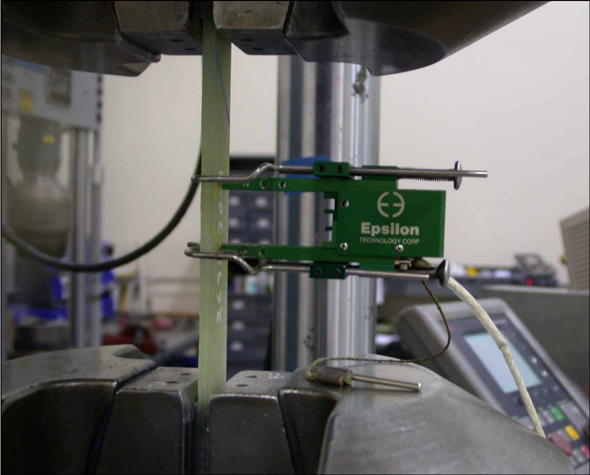
ASTM D3039 Mod. Test Setup at Intec
