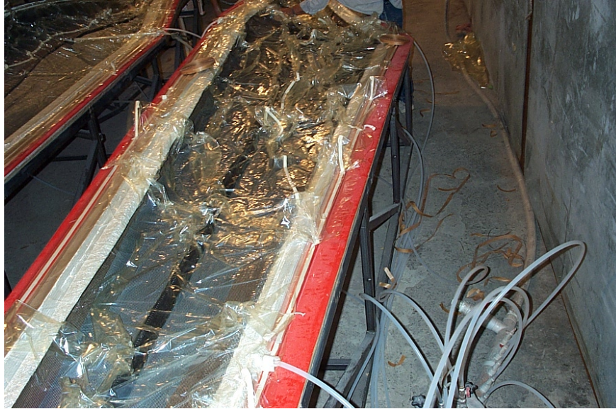
Figure 91 – BSDS Vacuum Bagging
