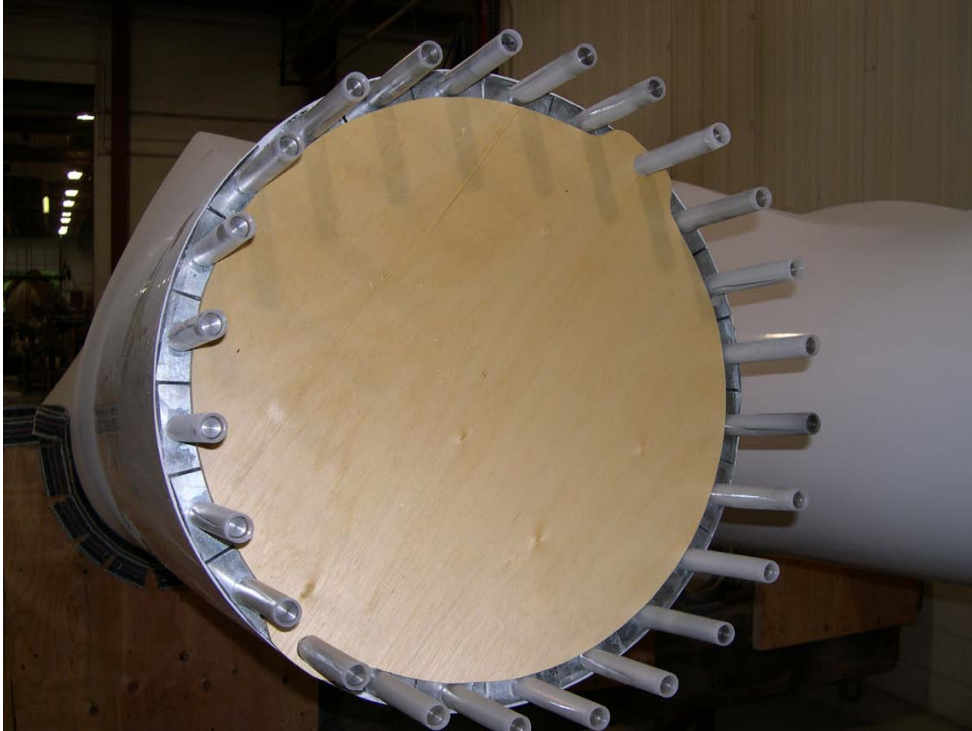
Figure 109 – BSDS Shipping Preparation
