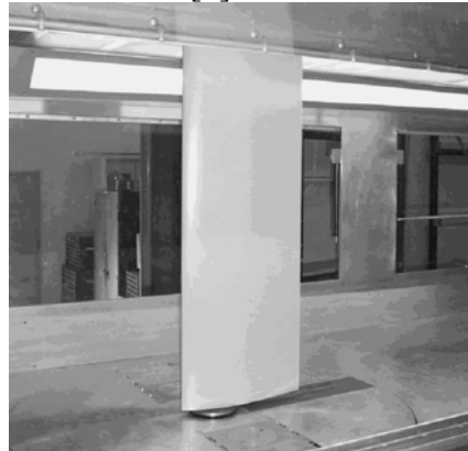
Figure 4. A two-dimensional airfoil model, mounted in the UCD AWT test section.
