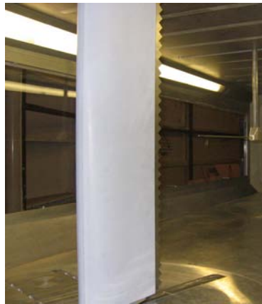
Figure 5. The FB3500-1750 airfoil model, with single 90°-serrated plate, mounted in the UCD AWT test section.
