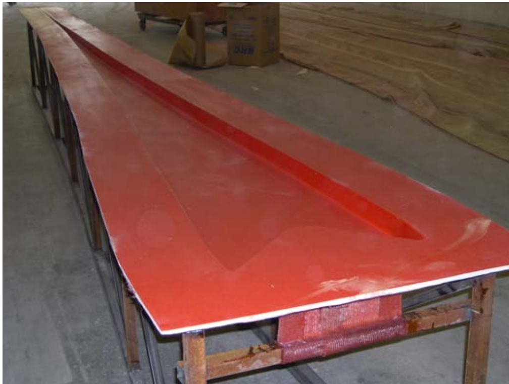
Figure 5 TX-100 Shear Web Mold
