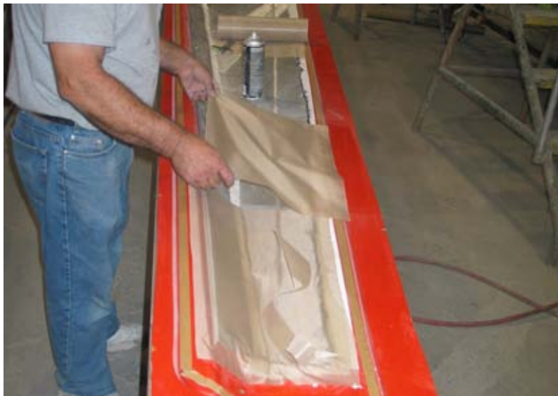
Figure 23 TX-100 Vacuum Bagging (1)
