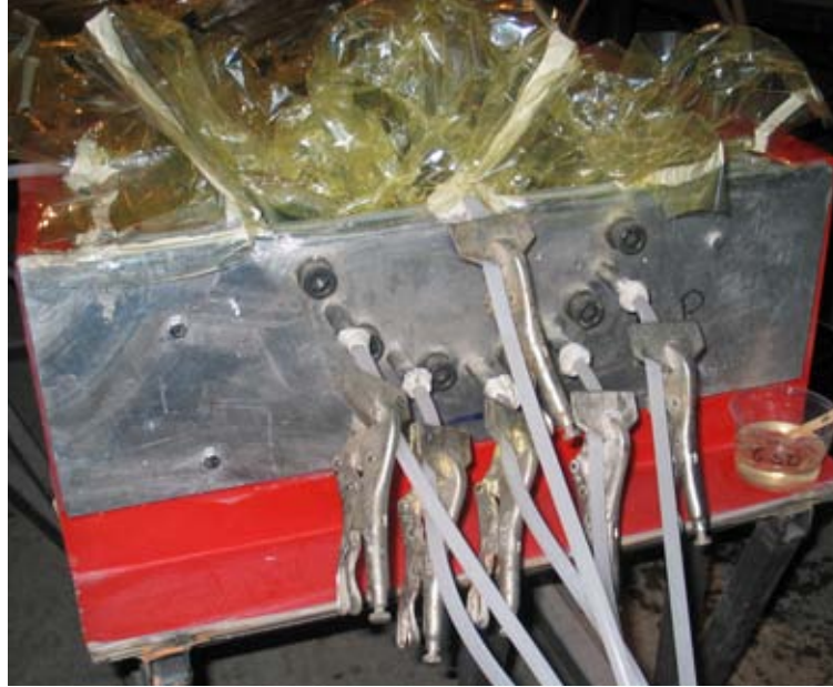
Figure 25 TX-100 Vacuum Bagging (3)
