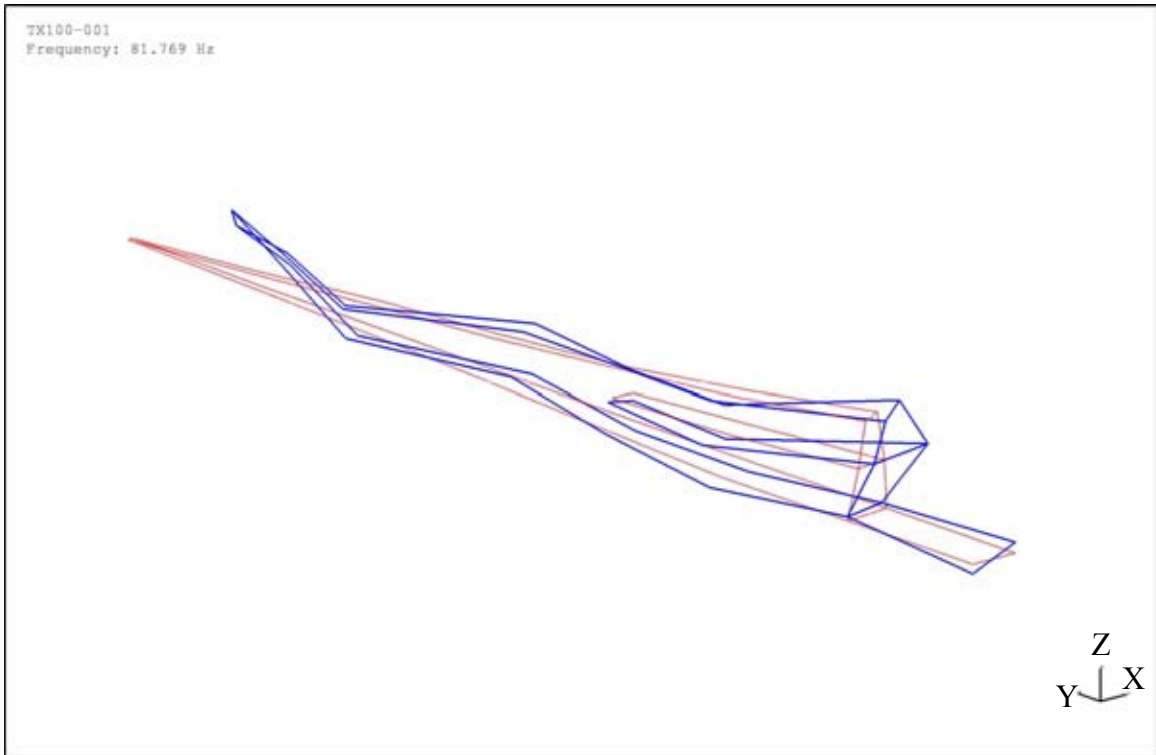
Figure A-10. Coupled Mode #2 ( f=82.13 Hz, \zeta = 0.50 %) Blade Serial #TX-100-001
