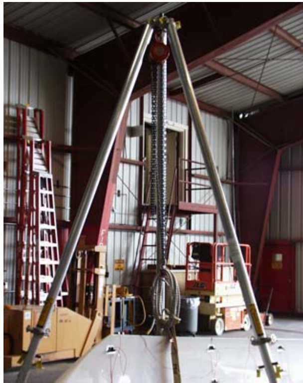
Figure C-19. Detailed view of the single-strap suspension system
