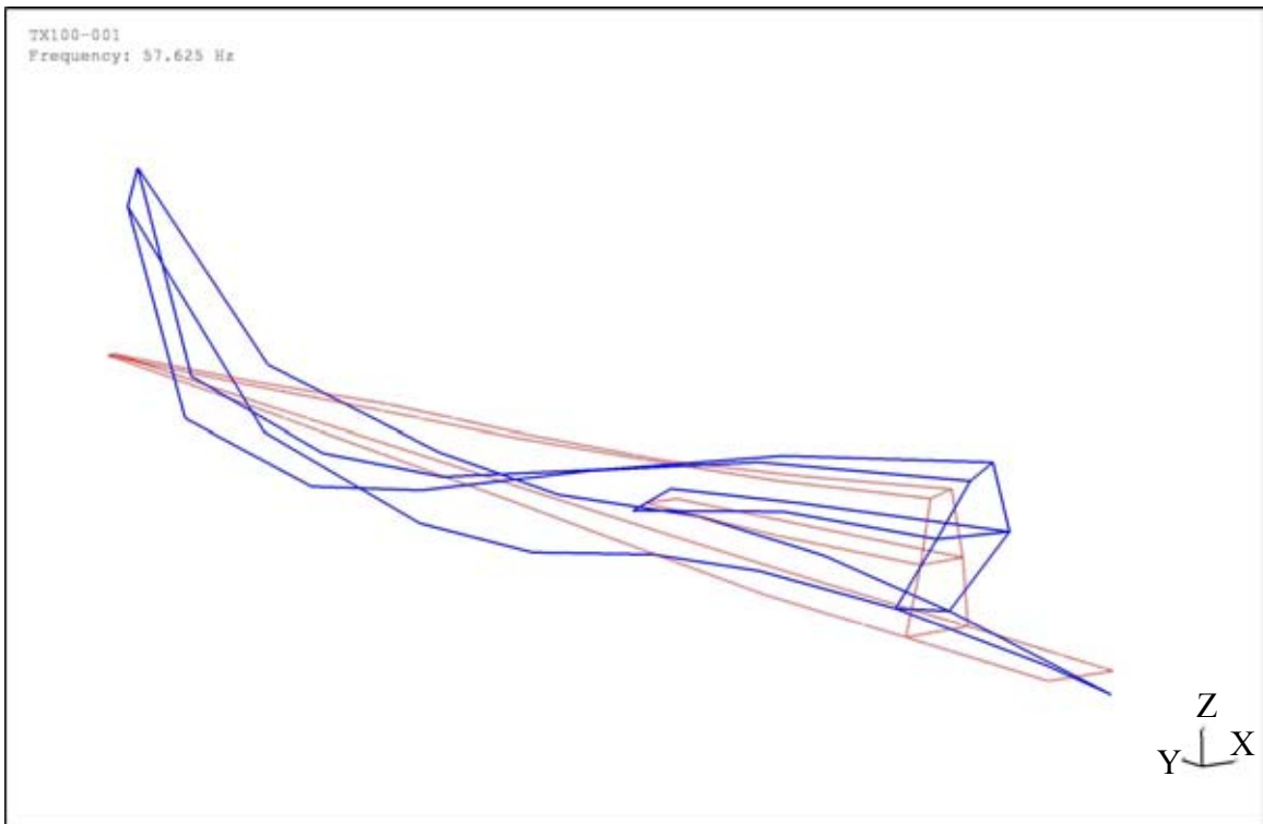
Figure A-7. First Torsional Mode ( f = 58.00 Hz, \zeta = 0.71 %) Blade Serial #TX-100-001
