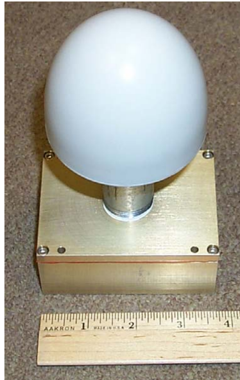
Figure 2-11. GPS Receiver/Antenna Configuration.
