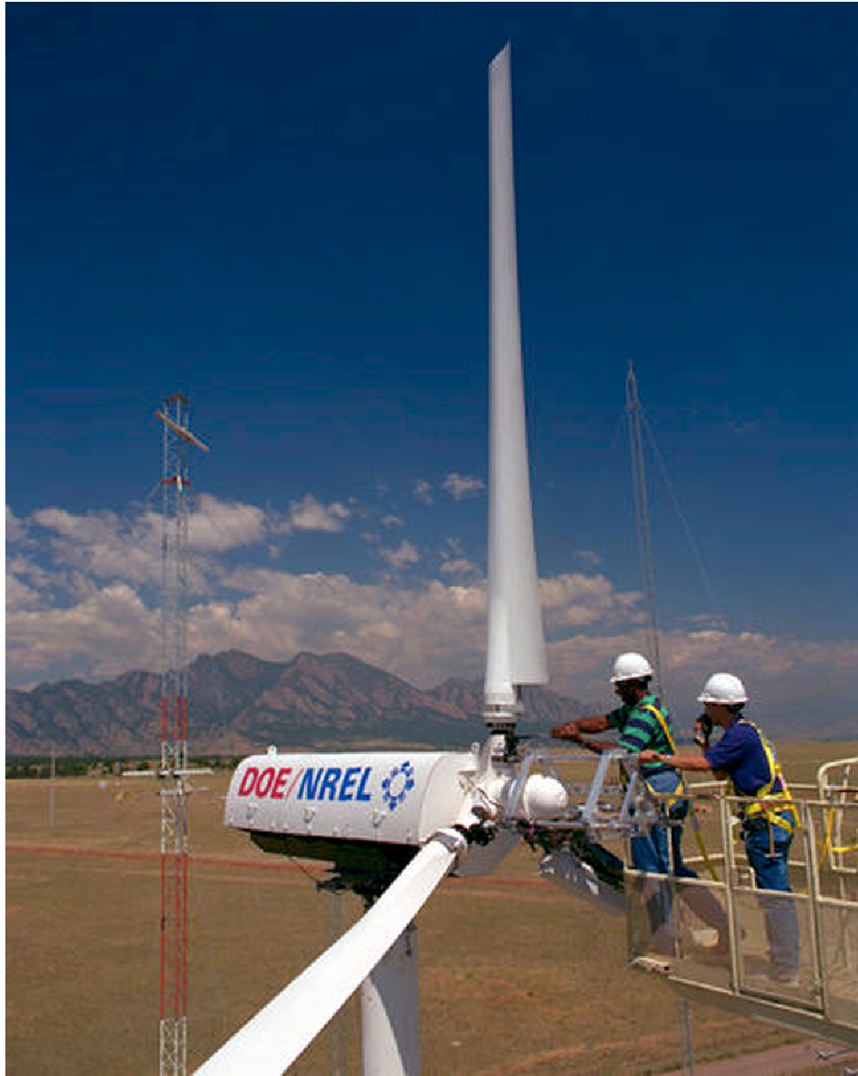
Figure 1.4: Close-up of DOE/NREL Unsteady Aerodynamics Experiment Phase III turbine installed at NWT. Photograph courtesy of the National Renewable Energy Laboratory, www.nrel.gov .
