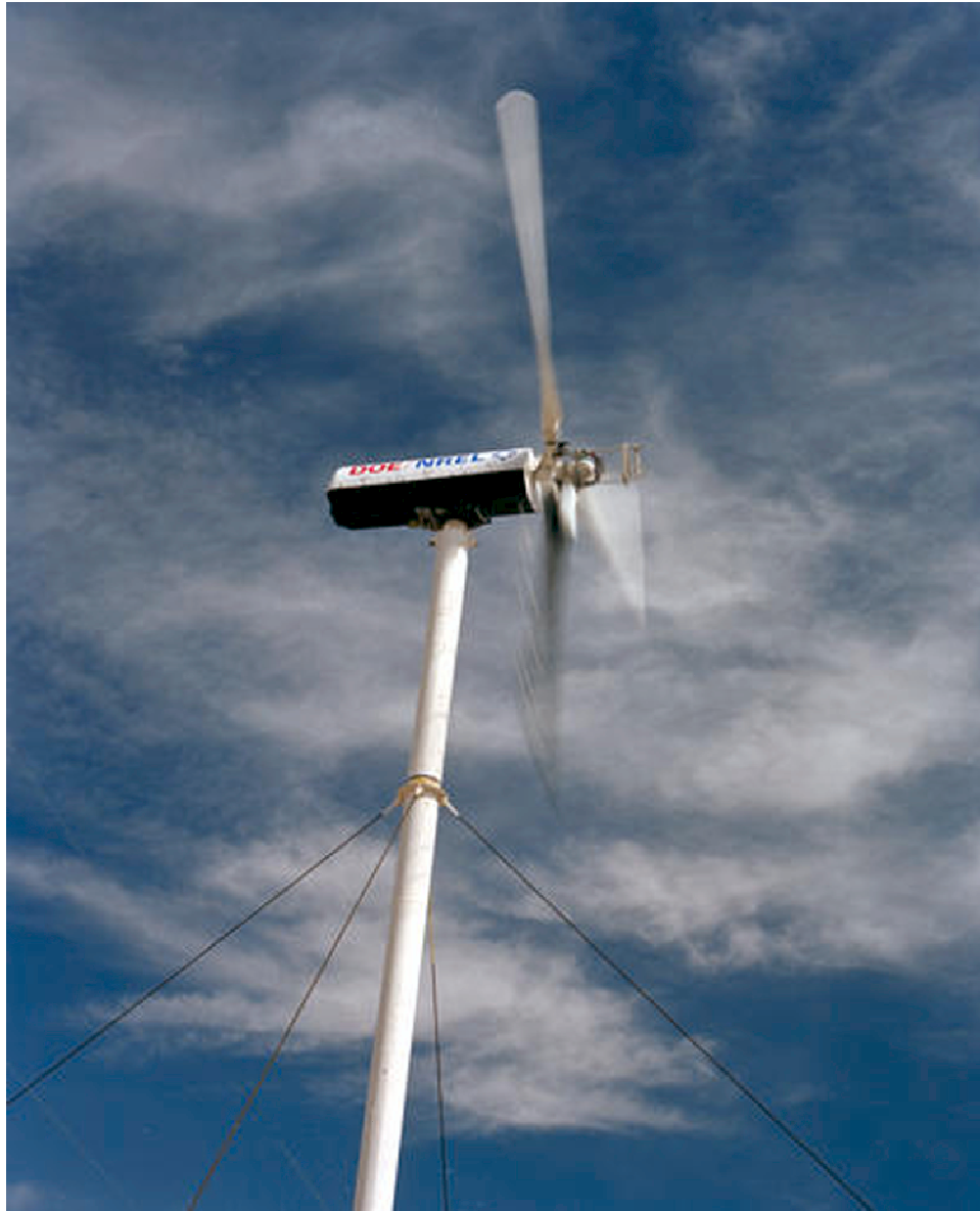
Figure 1.3: Department of Energy/National Renewable Energy Laboratory's Unsteady Aerodynamics Experiment Phase III turbine installed at the National Wind Technology Center. Photograph courtesy of the National Renewable Energy Laboratory, www.nrel.gov .
