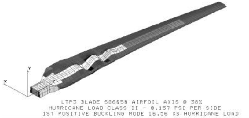
Fig. 5.9 - Hurricane Loads Buckling Shape – 1 st Positive Mode
