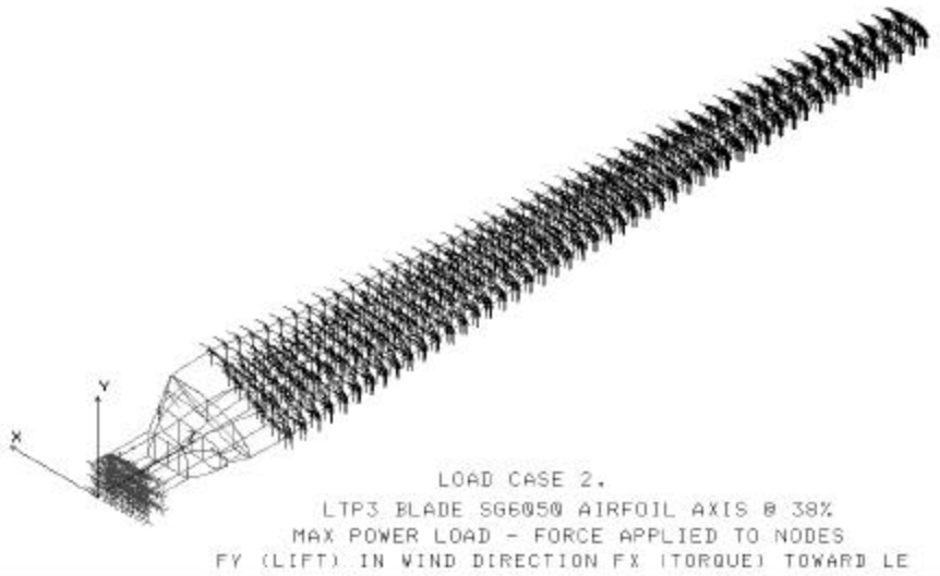
Fig. 3.7 - Max Power Load FEM Modeling – Final Design
