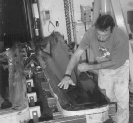
Fig. 4.4 - Open tool surface conditioning A FMI technician checks for surface blemishes. Note hinge detail and latches on the backside of the tool. Copper pipes on either side of the hinge are liquid inlet and outlet ports to heat or cool the tool during process or curing cycles.
