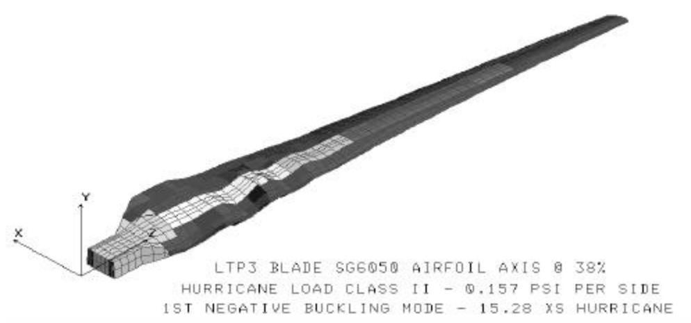
Fig. 5.8 - Hurricane Loads Buckling Shape – 1 st Negative Mode
