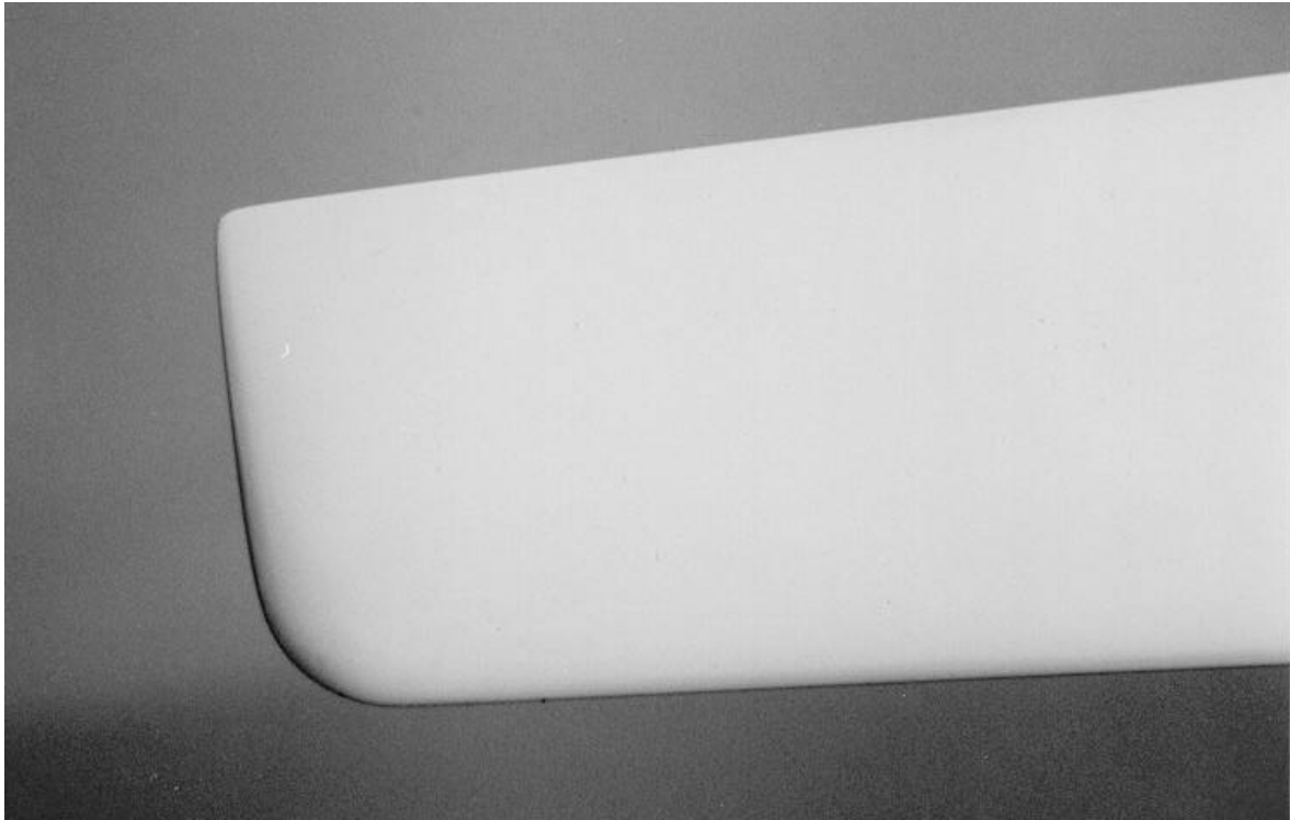
Fig. 4.10 - Tip Detail: Prototype blade tip, upwind side, after painting
