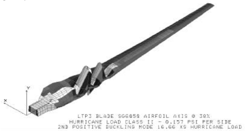
Fig. 5.10 - Hurricane Loads Buckling Shape – 2 nd Positive Mode
