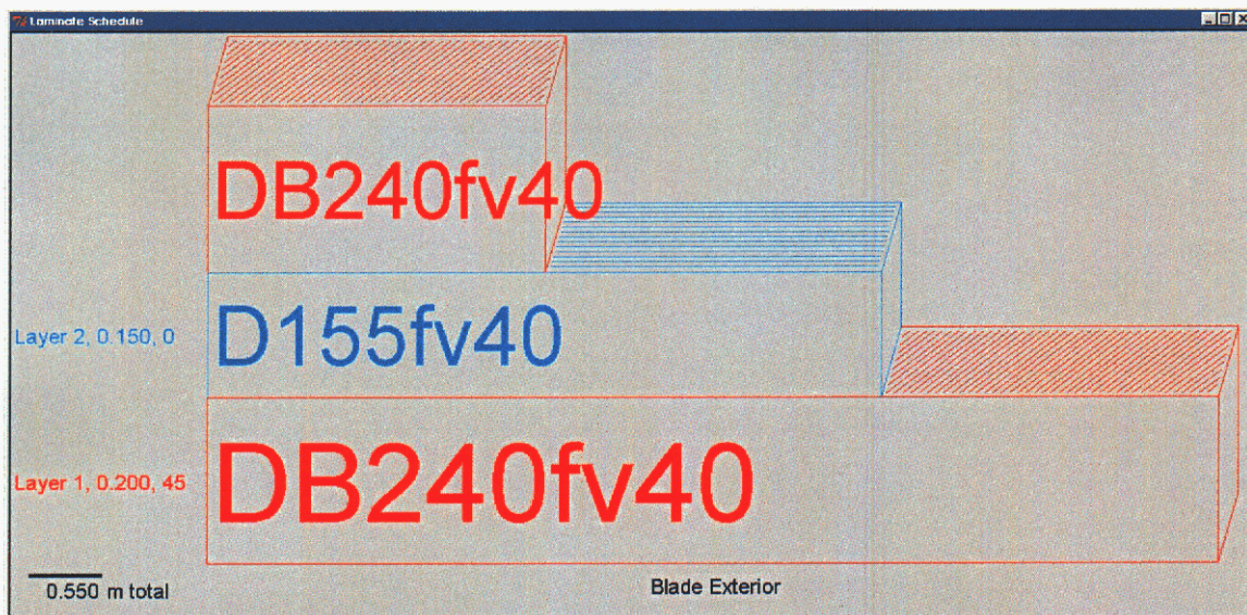
Figure 5.22 Schematic display of composite laminate material definition after two layers have been defined for an odd symmetric stack.
