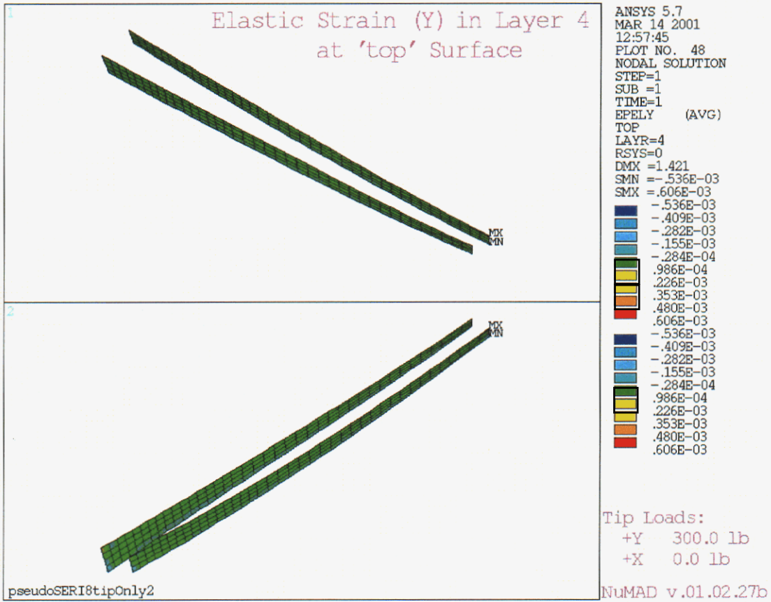
Figure 10.60 Automatically created image ShearWebLayer4topeY.jpg . Strains are in element Y directions at “top” surface of layer 4.
