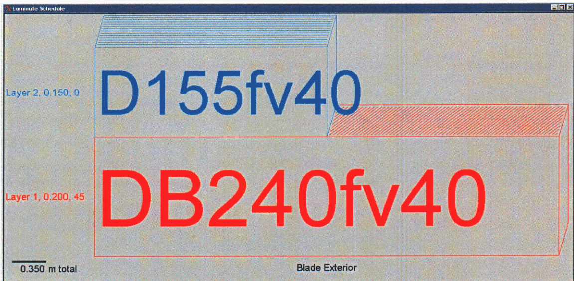
Figure 5.19 Schematic display of composite laminate material definition after two layers have been defined.
