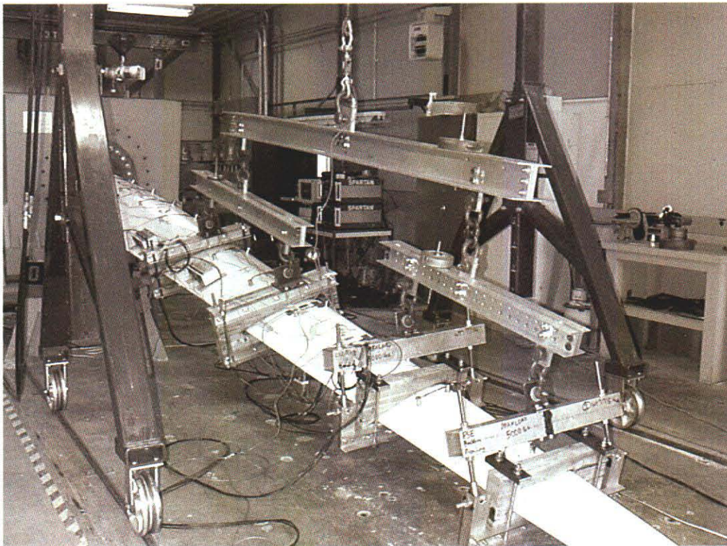
Figure 4.4 Photograph of the ERS-100 Blade in the Test Stand
