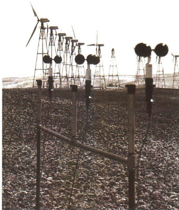
Figure 5. 4 Photograph of the Anemometer Calibration Frame.
