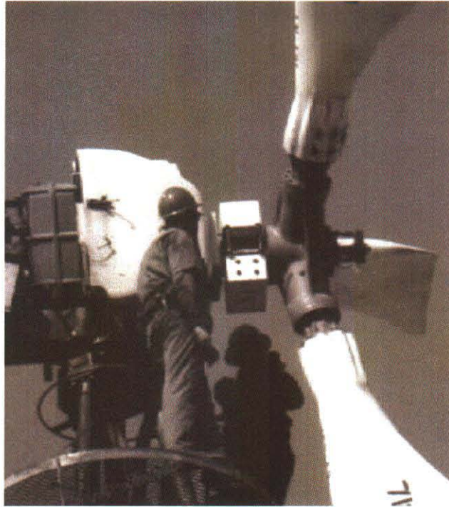
Figure 5. 8 Photograph of the Rotor Instrumentation
