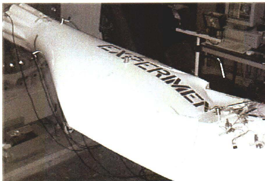
Figure 4.6 Photograph of the ERS-100 Blade After Static Failure
