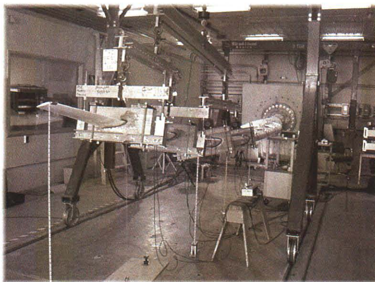
Figure 4.5 Photograph of the ERS-100 Blade Under Load
