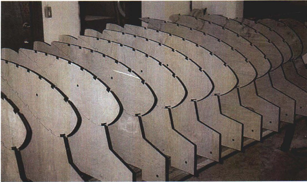
Figure 3.11 Photograph of ERS-100 Blade Pattern Templates
