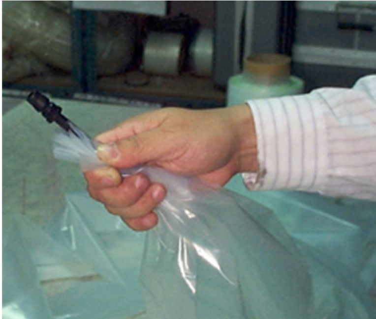
Figure 5.4a Place a Nozzle at the End of the Bag
