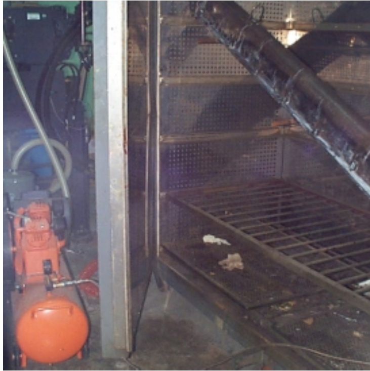
Figure 5.7 D-spar In Oven for Curing; Compressed Air Unit at Lower Left Corner
