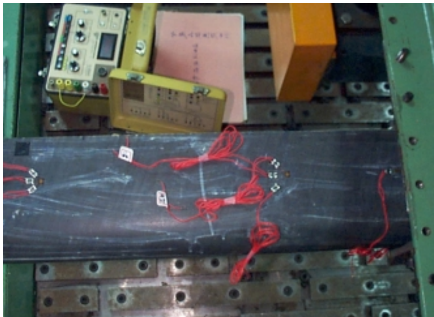
Figure 6.4 Strain Gauges Location at Top Surface
