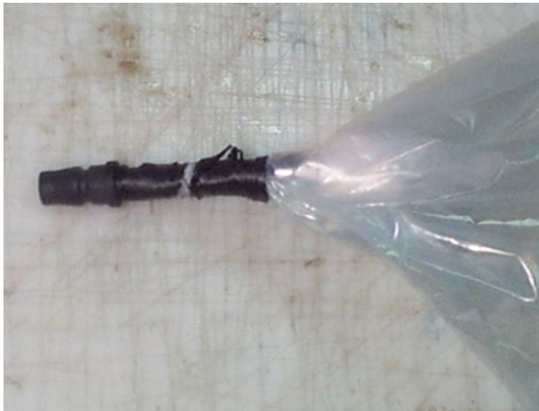
Figure 5.4b Strings of Prepregs Wrapped around the Nozzle for Sealing
