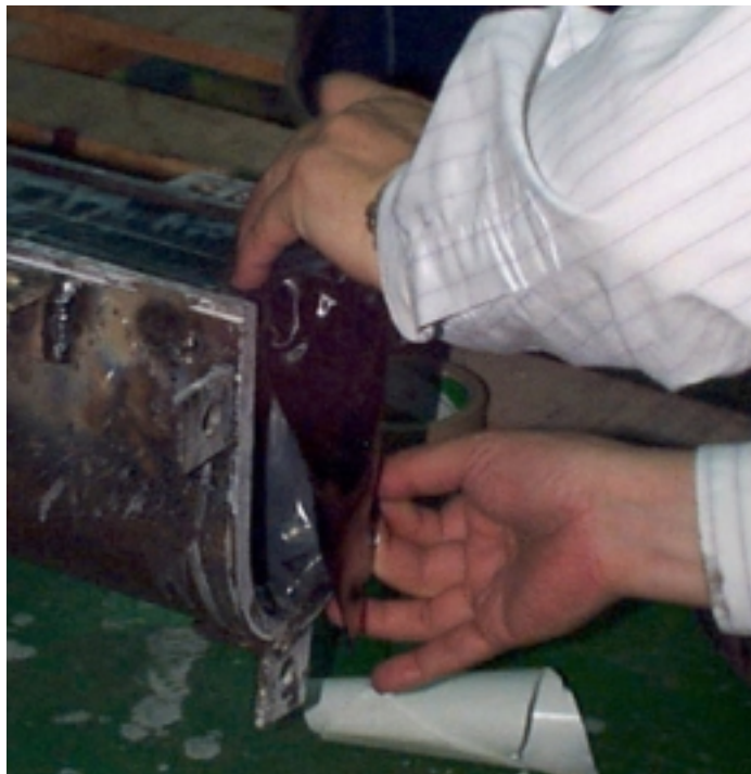
Figure 5.6 Protect Two Ends with a Sheet of [\pm 45^{\circ}_2]_T Laminate
