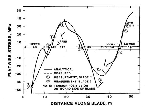
Fig. 12. Centrifugal Stress Distribution at 40 RPM
