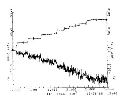
Fig. 10. Upper Root Flatwise Stress vs. RPM
