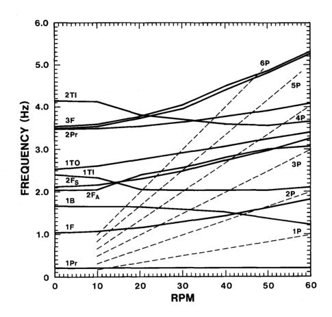
Fig. 7. Rotor Fanplot - Brakes Disengaged
