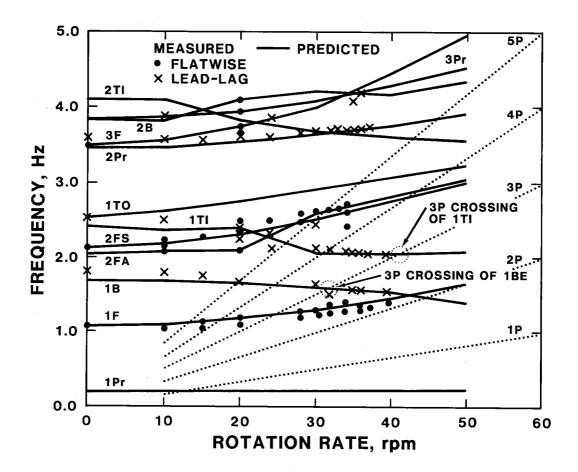
Fig. 9. Rotating Modal Frequencies - Measured vs. Predicted
