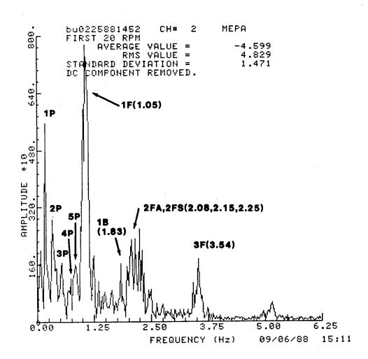
Fig. 8. Strain Amplitude Spectrum at 10 RPM
