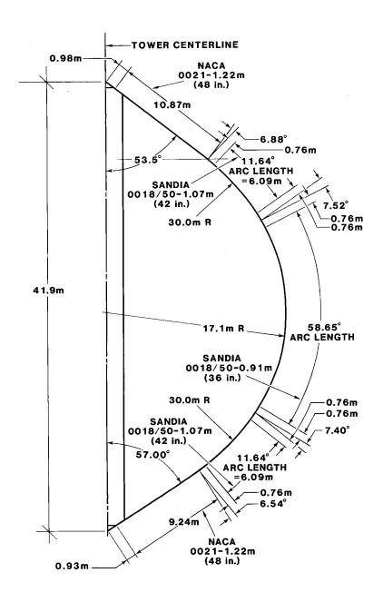
Fig. 2. Blade Shape Geometry
