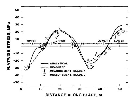
Fig. 11. Centrifugal Stress Distribution at 28 RPM
