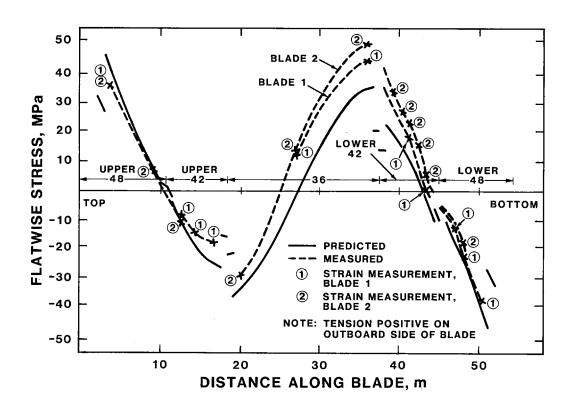
Fig. 4. Flatwise Gravity Stress Distribution
