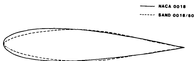
Figure 1. Comparison of NACA 0018 Airfoil Profile with SAND 0018/50
