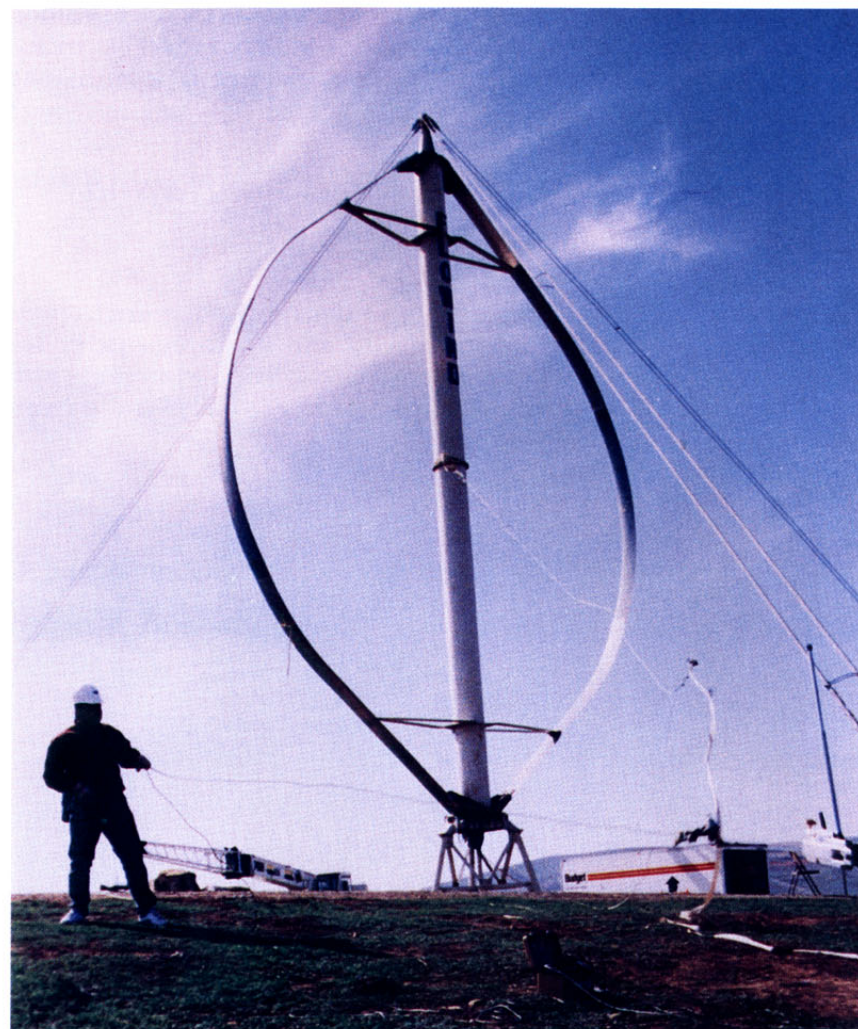
Release of cable by worker causes VAWT structure to vibrate. Instrumentation mounted on structure record these motions and send data to computer for analysis.
