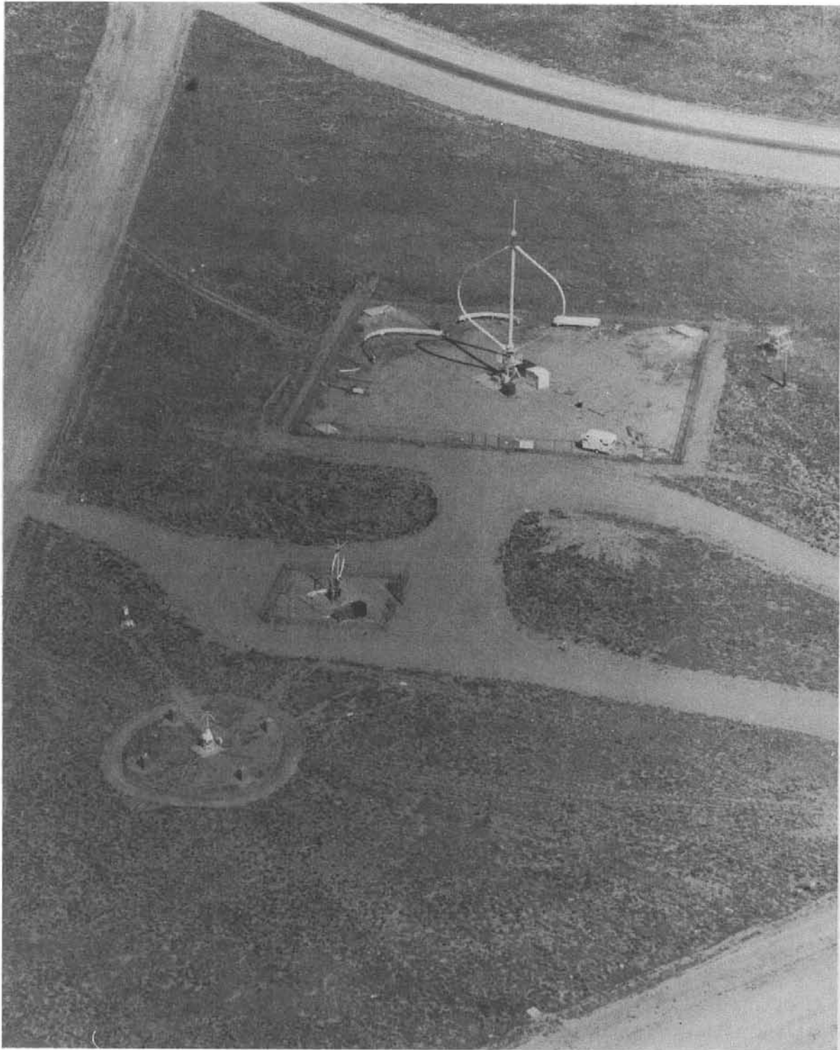
The Darrieus wind turbine generator research testing laboratory at Sandia National Laboratories. A view of the vertical axis wind turbines (VAWT) 2 meter, 5 meter, and 17 meter systems that are the primary lift-driven machines supporting the research and technology for the developing of large wind turbines for the United States Department of Energy.
