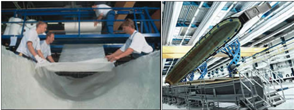
Figure 12: Images of the typical mold process (19).
