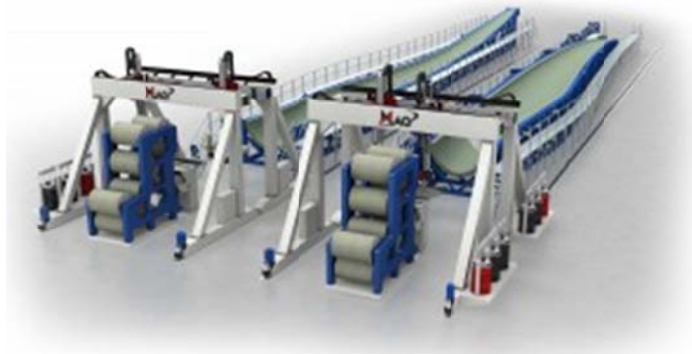
Figure 13: Automated blade manufacturing system (21)
