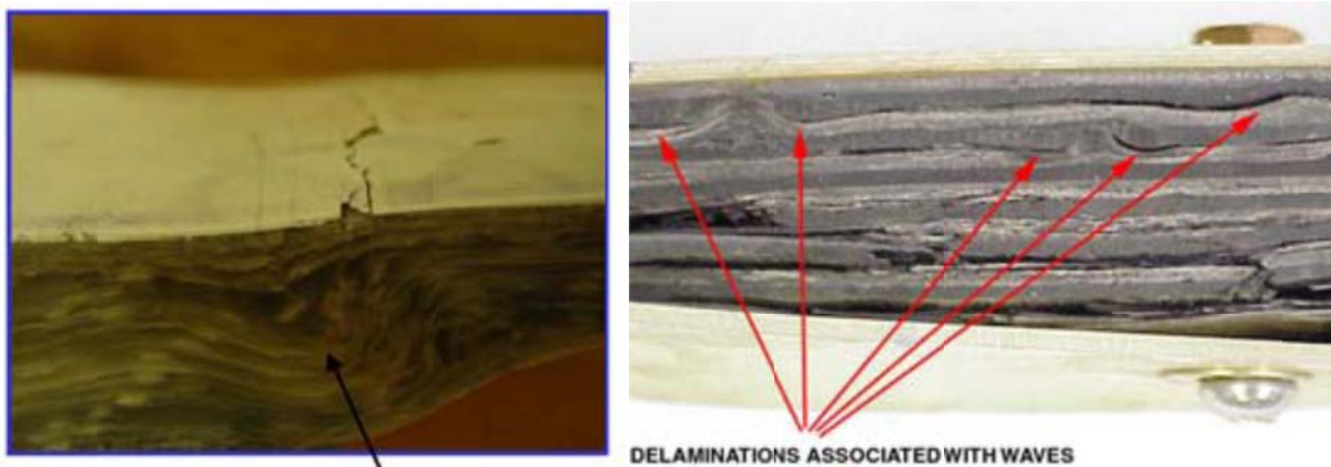
Figure 14: In-plane and out-of-plane waves and delaminations in composite materials and resulting failures (12).
