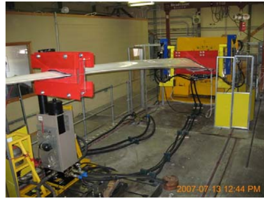
Figure 3. Fatigue testing of TX-100 blade at NREL's NWTC.
