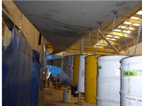
Figure 14. Static testing of first STAR blade.
