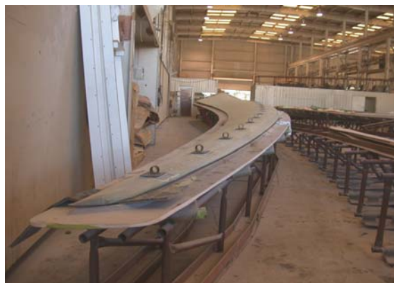
Figure 11. Fabrication of 1 st STAR Blade
