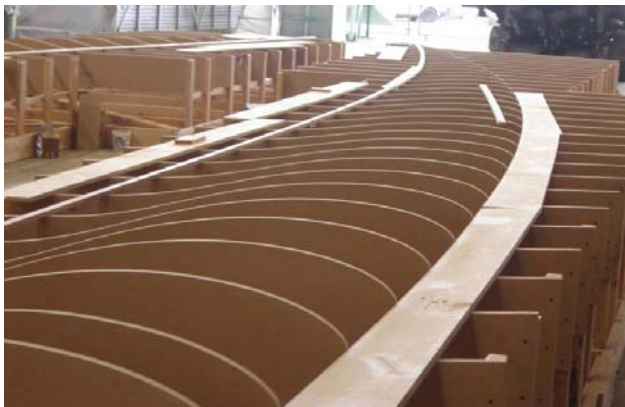
Figure 9. Fabrication of STAR Plug
