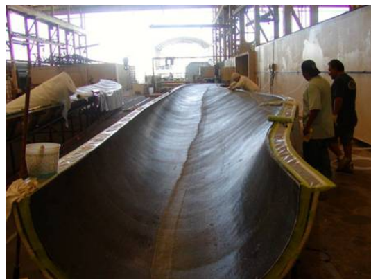
Figure 10. Lay-up of STAR Blade
