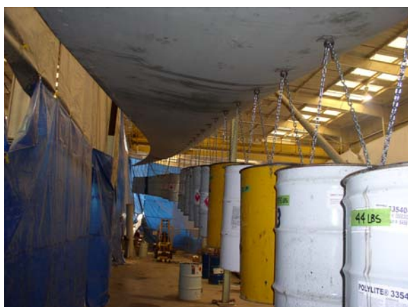
Figure 13. Static Testing of 1st STAR Blade
