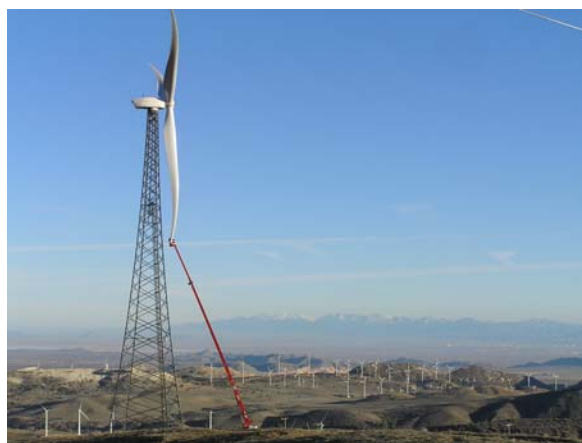
Figure 22. STAR Blades Mounted for Flight Testing
