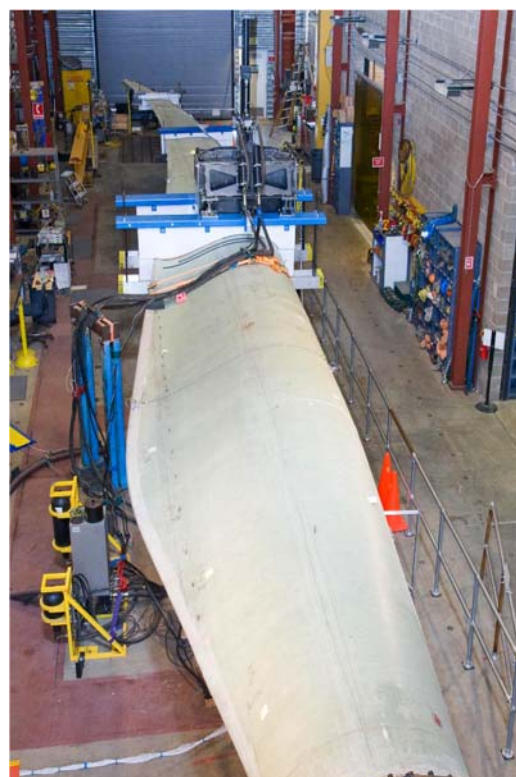
Figure 14. STAR prototype blade in NREL test stand with loading saddles.
