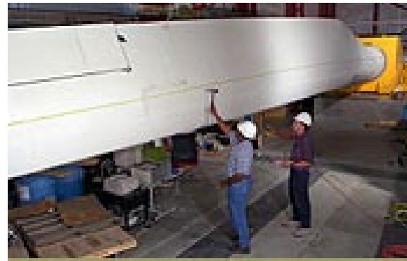
Figure 3: Wind turbine blade with trailing-edge flap in test stand (Courtesy of National Renewable Energy Laboratory)
