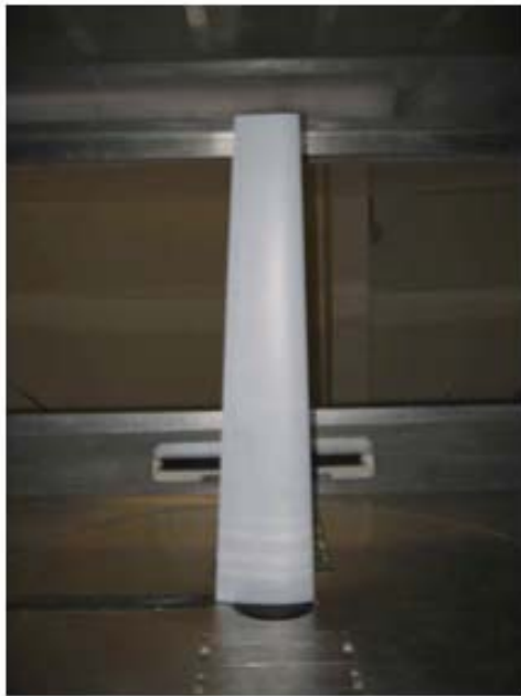
Figure 7: Blade tip model mounted in wind tunnel test section. Flow from right to left. Model span is 24.7 inches.
