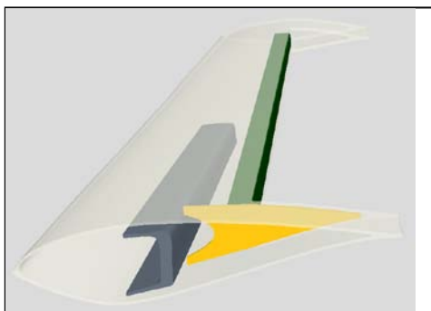
Figure 3 Modifications to the Outboard Blade to Accommodate Trailing Edge Load Control Modules. Dark Gray is Existing Shear Web, Green is Retrofit Aft Shear Web, Yellow is Retrofit Rib (View is Looking Outboard From 7.0 m).
