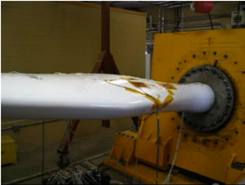
CX-100 Dimple (left) and Tip Movement (right) at Failure
