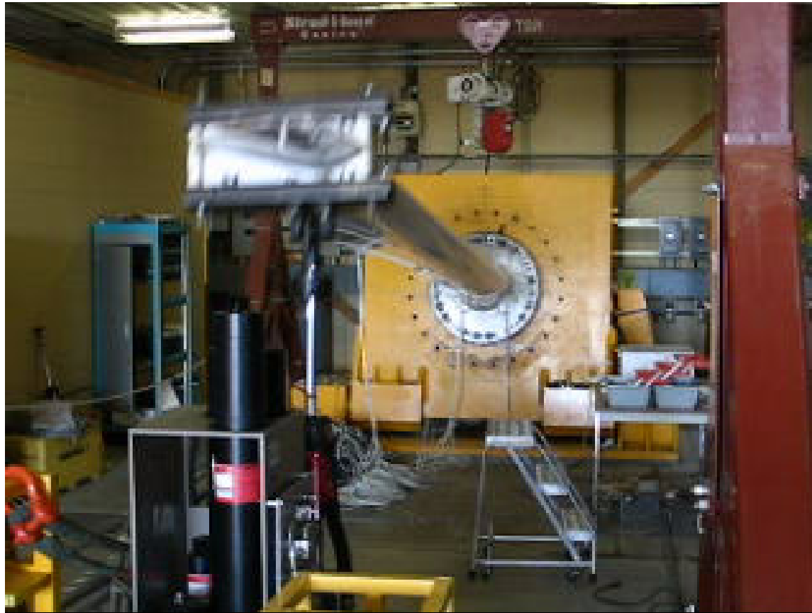
CX-100 Early in Fatigue Test
