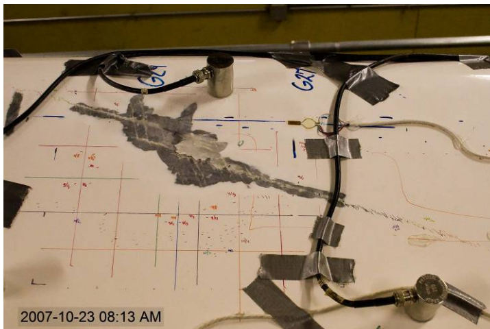
Figure 18: TX-100 high-pressure skin damage area.
