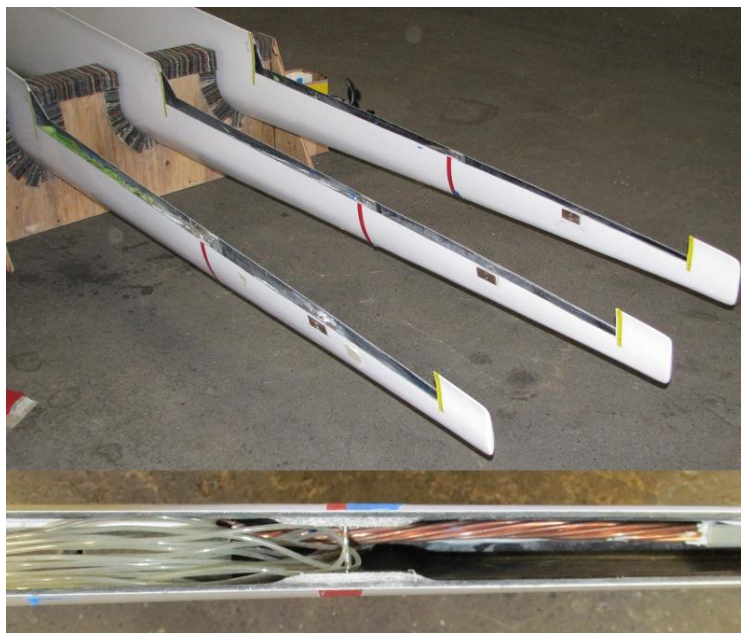
Figure 4. Top: blade set after removal of 6-foot section. Bottom: close-up of cavity showing surface pressure tap tubing and lightning cable.
