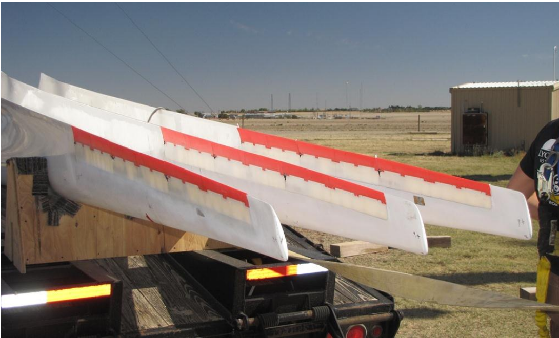
Figure 6. Fully assembled SMART blade set.
