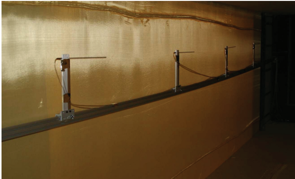
Figure A.1. Photograph and diagram showing the system of Pitot static tubes used to measure the pressure distributions over the inside of the Kevlar acoustic windows, adapted from Crede [8].
