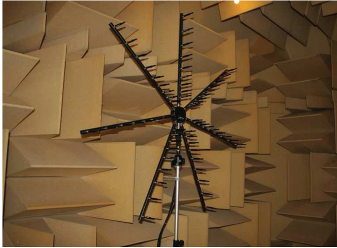
Figure 17. View from inside the port-side anechoic chamber showing microphone phased array.
