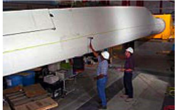
Fig. 3-5 Wind turbine blade with trailing-edge flap in test stand. (Source: NREL 6 )
