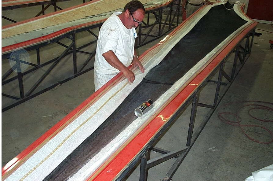
Figure 67 CX-100 Vacuum Bagging (3)
