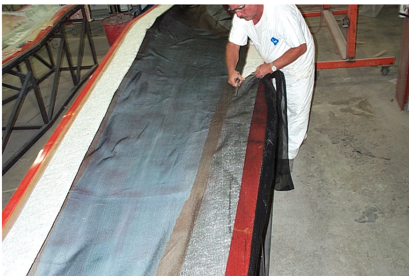
Figure 66 CX-100 Vacuum Bagging (2)
