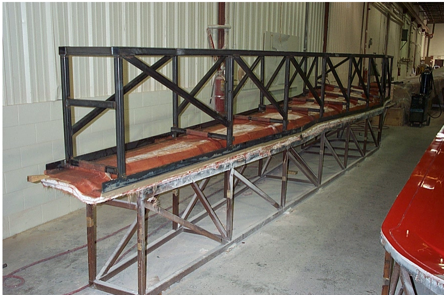
Figure 27 CX-100 Steel Mold Bracing (1)
