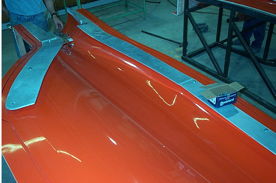
Figure 32 CX-100 Mold Flanges (1)
