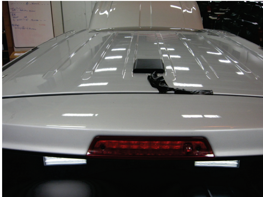
Figure 4-50 Antenna Mounted on POC Vehicle
