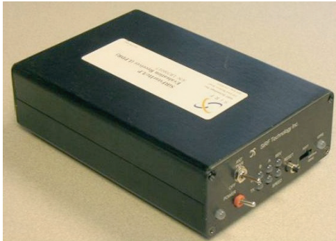
Figure 4-52 SiRFStar Positioning Unit
