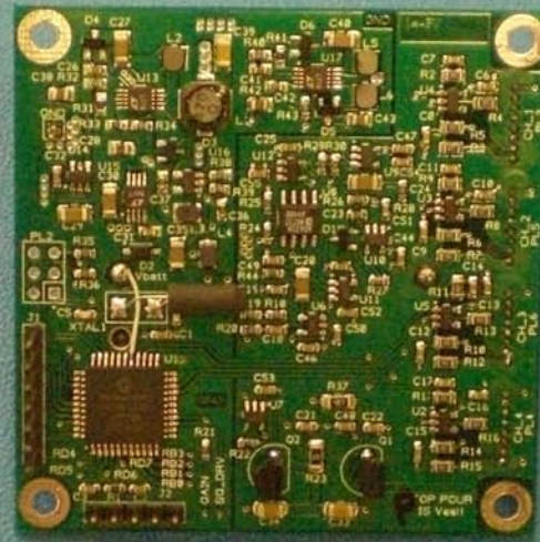
DSP Board (Inside EFM)
