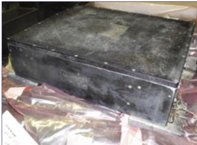
Figure 3.6-1. The Modular Auxiliary Data System recorder, found near Hemphill, Texas. While not designed to withstand impact damage, the recorder was in near-perfect condition when recovered on March 19, 2003.
