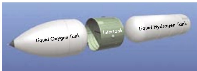
Figure 3.2-1. The major components of the External Tank.
