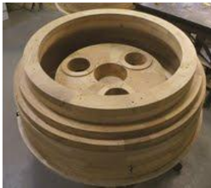
Wood pattern for a cover plate in the drive reduction housing for a gas turbine engine used by Solar Turbines.
