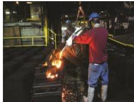
Pouring metal to produce iron castings.
