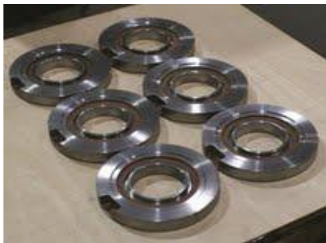
Bearing Retainer Ring Castings (Weighing 29 lbs each)
