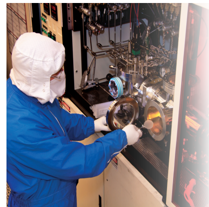
Technologist Jeff Kempisty of SNL removes an InGaN LED wafer from the Veeco MOCVD system.
