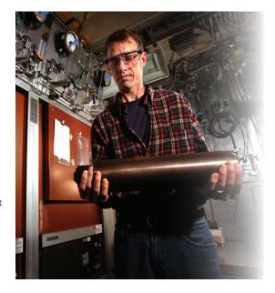
Brian Somerday, an SNL researcher, prepares to load a hydrogen pressure vessel into a laboratory furnace.
