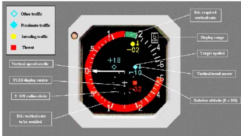
Figure 16 TCAS RA Display implemented on an IVSI
