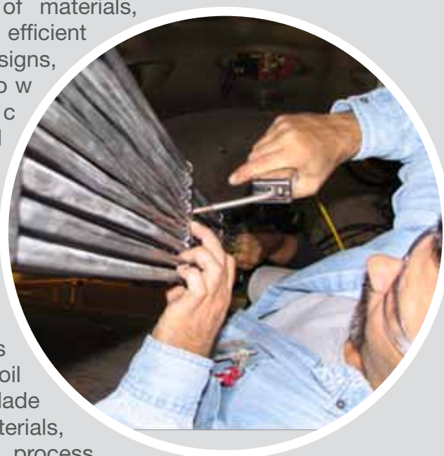
Sandia researchers prepare a mock-up of a spent nuclear fuel rod bundle for testing.
