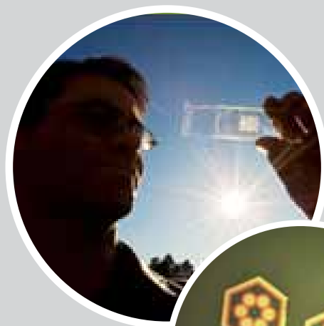
Greg Nielson holds up a test strip of the solar glitter cells. To the right is a micrograph of the crystalline silicon micro-PV cells.
