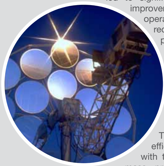
An early version of the dish-Stirling concept used many small cast parabolic mirrors.
