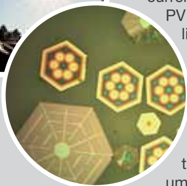
Greg Nielson holds up a test strip of the solar glitter cells. To the right is a micrograph of the crystalline silicon micro-PV cells.
