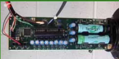
Teledyne power management package.
