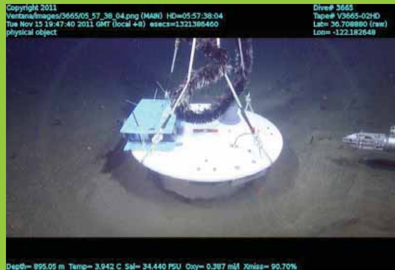
MFC after being pushed into sediment with Remotely Operated Vehicle manipulator. Courtesy Oregon State University.
