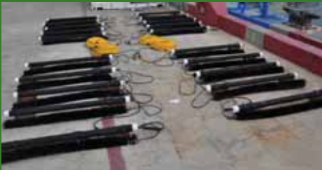
Anodes (black cylinders above) used to generate power for a stationary acoustic array used for surveillance.
