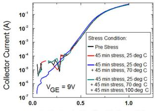
Collector to Emitter Voltage (V)
