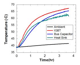
Figure 7. Temperature traces for (1) Ambient, (2) IGBT, (3) Bus capacitor, and (4) Heat sink for an operating, 700 W, single-phase inverter.
