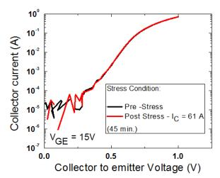
Figure 1. Pre and post-stress  $I_c$ -V<sub>CE</sub> curves for typical IGBTs, after 45 min stress at  $I_c \approx 61$  A.
