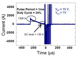
Figure 5. IGBT collector current resulting from pulsed gate input. Measurement is made at room temperature.
