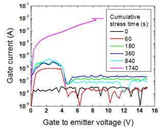
Figure 4.  $I_G$ -V<sub>CE</sub> curves resulting from stressing an IGBT at V<sub>GE</sub> = 20 V, V<sub>CE</sub> = 2 V ( $I_C \approx 38$  A), corresponding to a condition of high electric field in the gate oxide and moderate thermal stress.
