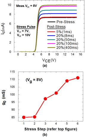
Figure 6. (a) DC I<sub>C</sub>-V<sub>CE</sub> curves for an IGBT subjected to increasing increments of AC stress. (b) The output conductance ( $g_0$ ) measured at the end-point of each of the curves in the top portion of the figure (V<sub>GE</sub> = 8 V, V<sub>CE</sub> = 15 V) for each of the steps in the sequence.
