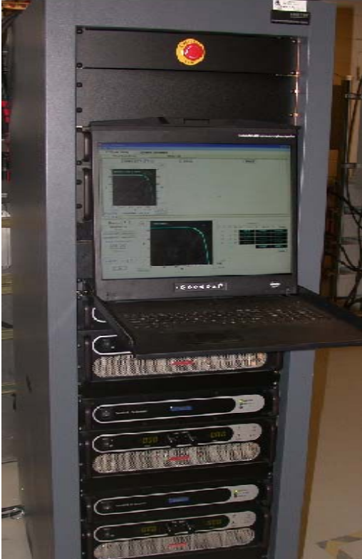
Fig. 1: Rack-mounted AMETEK PV simulator.
