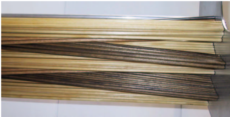
Figure 6.36: A photo of the \frac{1}{3} scale model of the straw-tube chamber. The picture shows the two directions of stereo wires as well as the straight wires.
