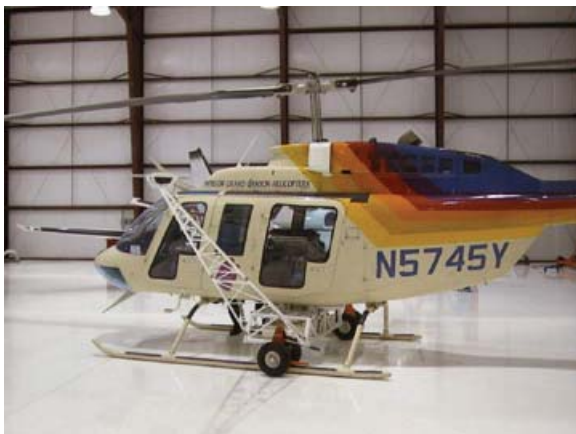
Figure 12. Photo. Dual GPS antenna and LiDAR system mounted on helicopter.
