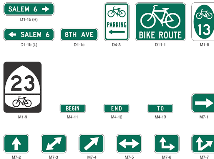
Figure 35: Bicycle Route Sign MUTCD (FHWA, 2003).
