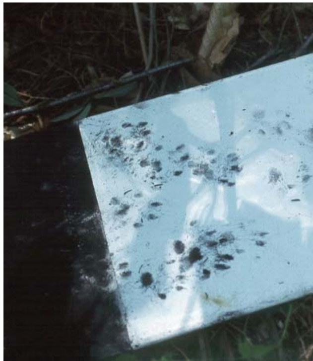
Figure 77. Photo. Sooted track plate with tracks of small and medium-sized mammals (Credit: Robert Long/WTI).
