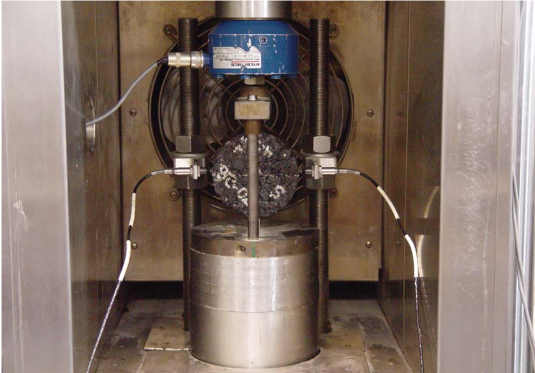
Figure 13. Photo. Diametral Resilient Modulus Test.
