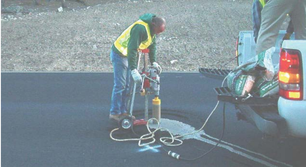
Figure 20. Photo. Typical Coring Operation by CFLHD Staff.
