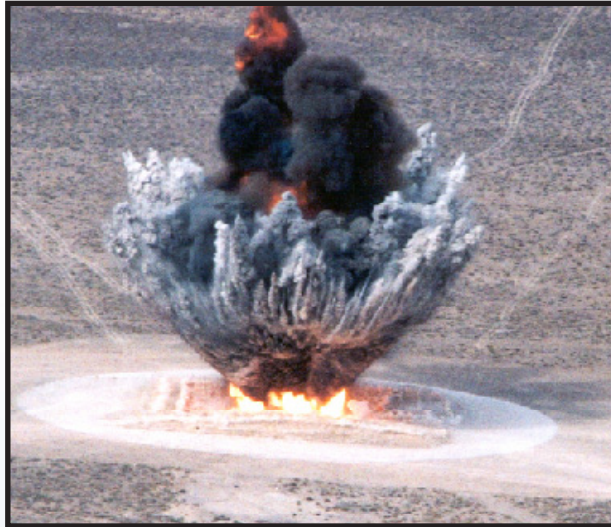
WATUSI is one of the largest activities conducted at BEEF by Los Alamos National Laboratory. The 36,600 pound TNT-equivalent, research and development activity was designed to validate low-end detection capabilities associated with ground motion and the acoustic footprint of an explosives detonation.
