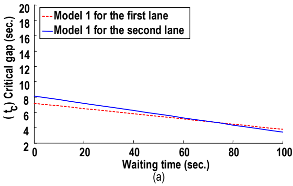
Figure ES.1 Effect of Waiting Time and Rain Intensity on Critical Gap Value for Different Models
