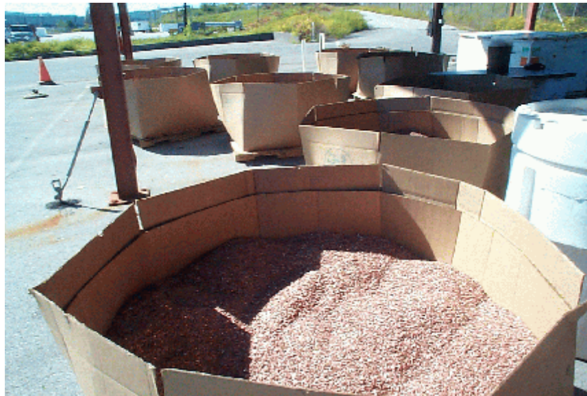
Figure 4.2: Containers of copper chop (recently surveyed using the conveyORIZED survey monitor)
