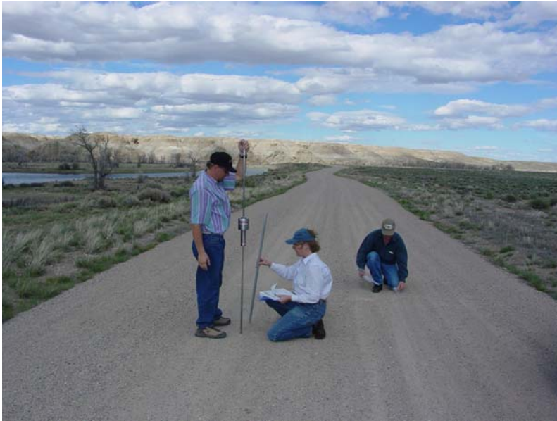
Figure 26. Photo. DCP testing.
