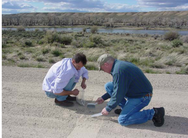
Figure 25. Photo. Sampling for Silt Load Test.
