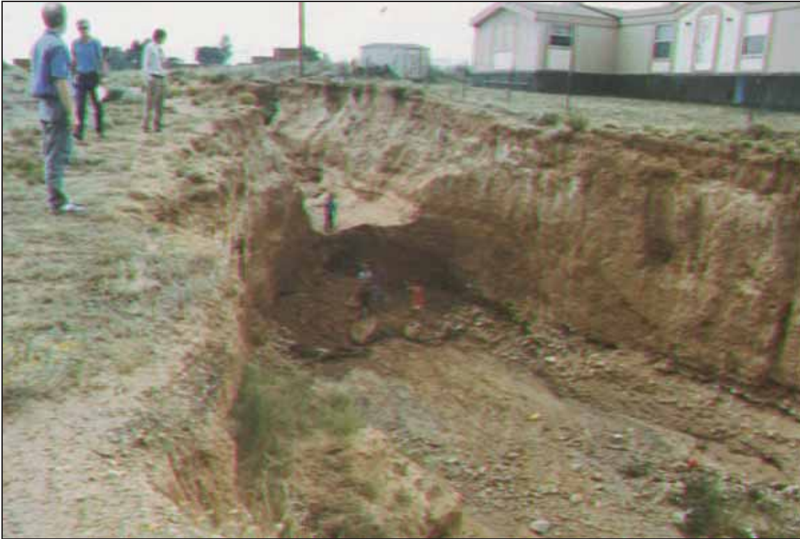
Figure 13. Photo. Example of head cut that can be expected to move upstream over time. (7)
